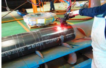
fabrication in process: Gas cutting
